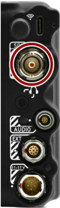
Figure: Front face of the 12G-SDI male BNC connector (looking at the back of the camera).
