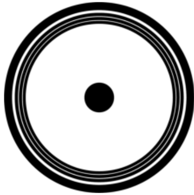
Figure: Front face of the female RP SMA port (looking at the back of the camera).
