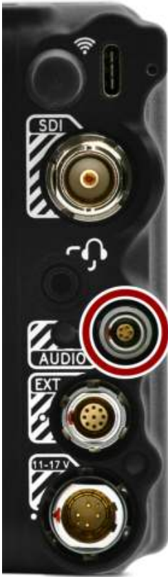
Figure: Front face of the female 5-Pin 00B audio connector (looking at the back of the camera).
