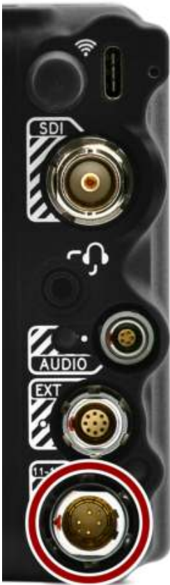
Figure: Front face of the male 6-Pin 1B DC power input connector (looking at the back of the camera).
