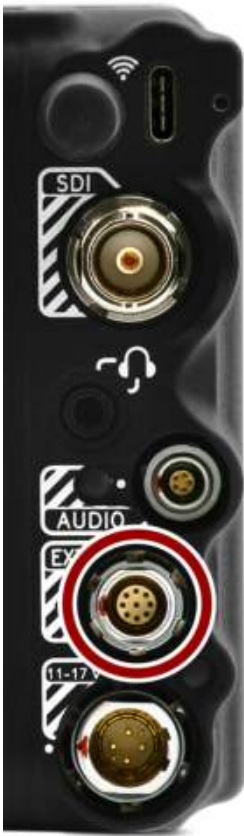
Figure: Front face of the female 9-contact Extension port (looking at the back of the camera).
