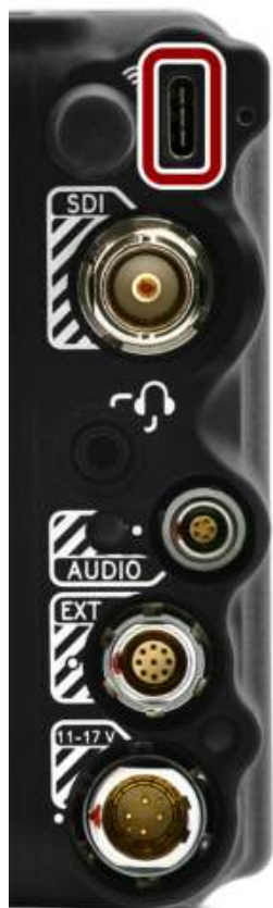
Figure: Front face of the USB-C port (looking at the back of the camera).
