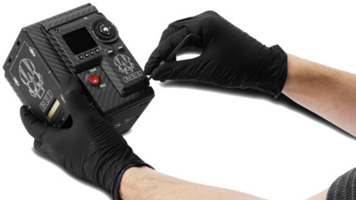
Figure: Reinstall the Side Module/Panel
