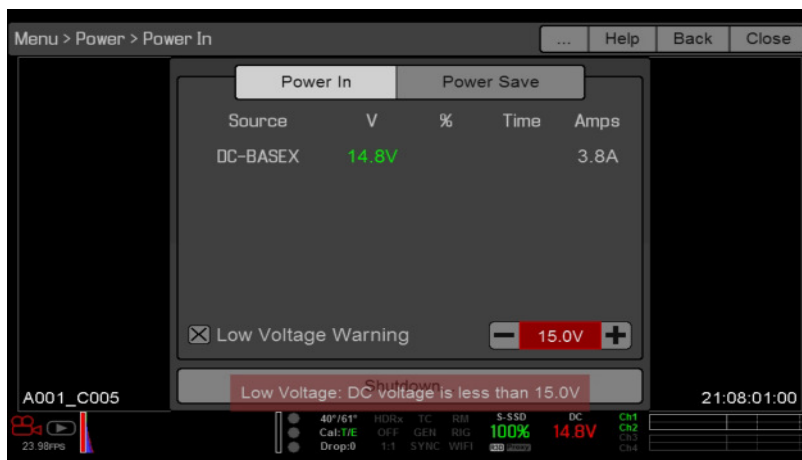
Figure: Low Voltage Warning
