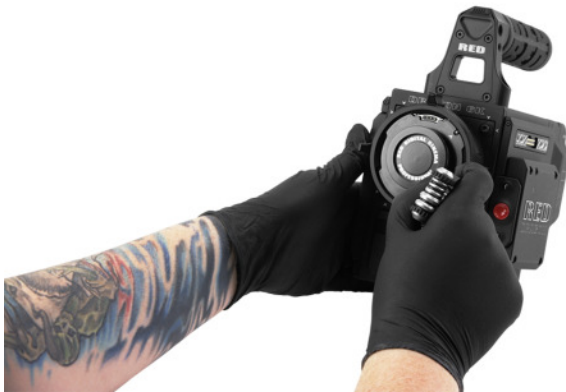
Figure: Remove the Lens Mount Screws
