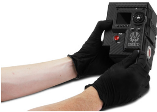
Figure: Remove the Side Module/Panel
