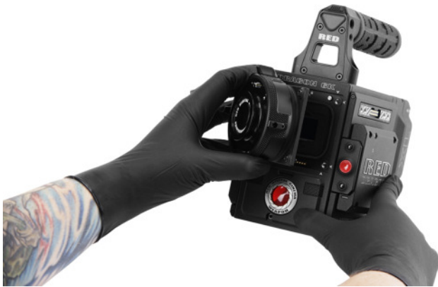
Figure: Align Lens Mount Pins
