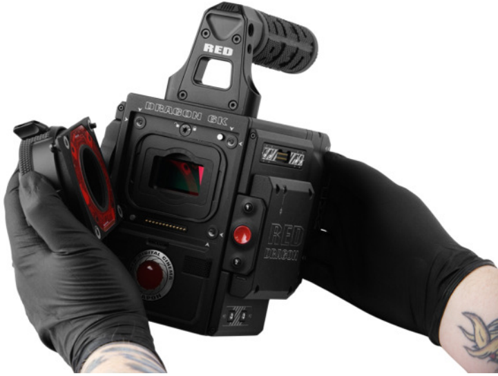
Figure: Remove the Lens Mount
